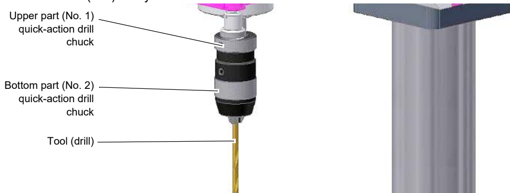
Img. 4-16: Quick-action drill chuck
