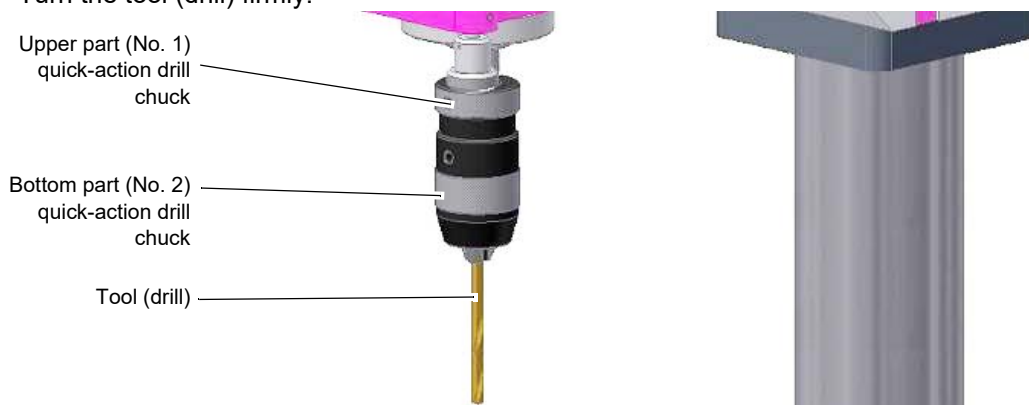
Img. 4-6: Quick-action drill chuck
