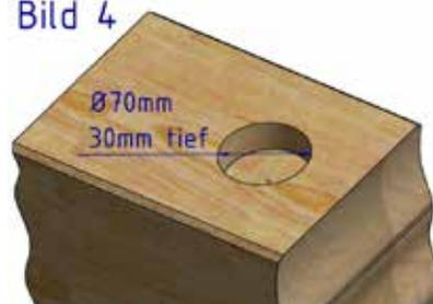
The milled slot for the coupling head must be created to the dimensions shown in Figure 4 using a Forstner bit or chain mortiser.
