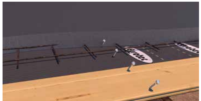
Layer structure, wood-concrete composite ceiling
