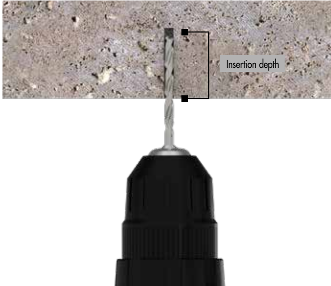
Step 1: Drill a hole with a 6 mm diameter.
