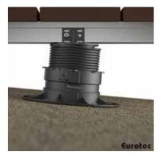
If there is risk of impact vibration on the decking, the decking pedestals should be secured in place. In addition, decking pedestals that are frequently subject to stresses should be secured by screws to avoid twisting.
