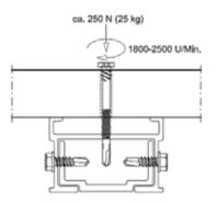
The screwing process should be finished when the screw head lies flush with the decking board surface.
