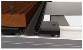
2 Maintain the clearance between the joints and lay the next floorboard.
