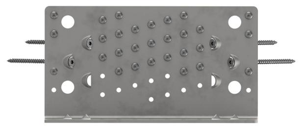
Figure B.18 Fastener Pattern Partial 2 for Shear Angle 240x230 and Shear Plate 230x120 in timber to timber connections (Symmetrical hole-pattern for both flanges)
