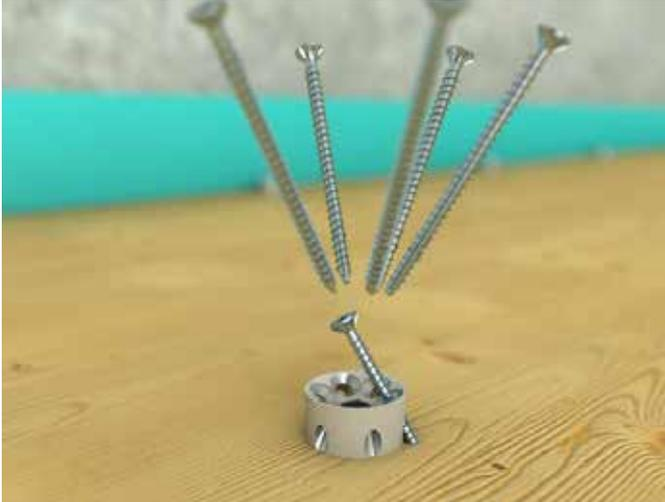
Step 3: Install the six KonstruX screws 6,5 mm x 100 mm in each hole of the steel cylinder, tightening one by one uniformly to prevent moving the cylinder out of position.
