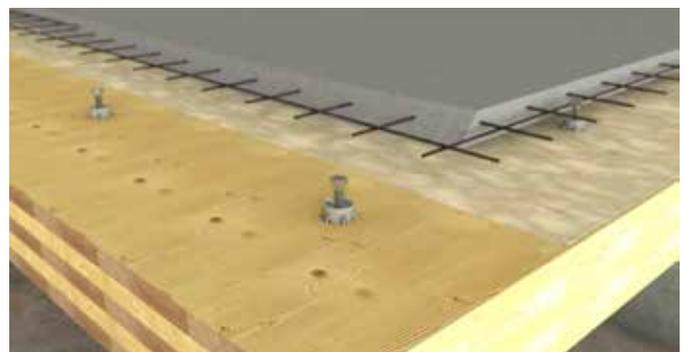
TCC MAX application for connecting CLT.
