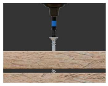
Without prior fastening, the screwing process creates a gap between the components.
