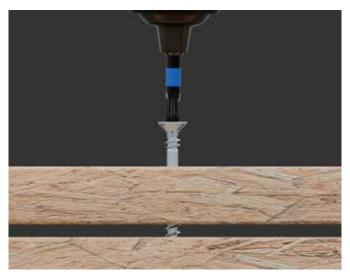
Without prior fastening, the screwing process creates a gap between the components.
