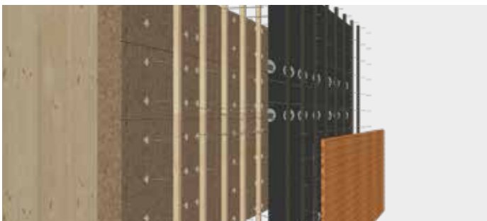
Fastening a façade using vertically positioned wooden slats and Topduo roof construction screw
