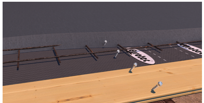
Layer structure, wood-concrete composite ceiling
