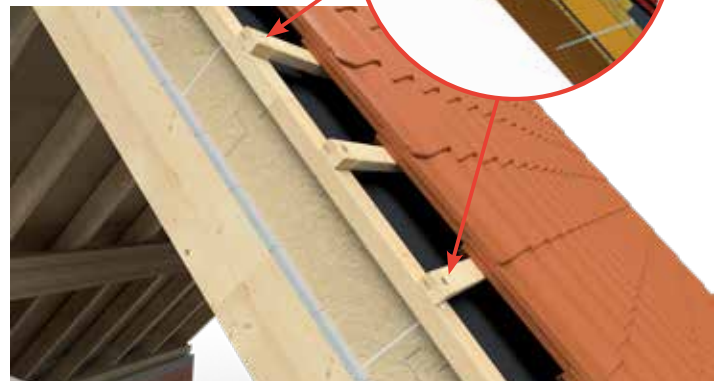
Wood-wood connections (rafter-level insulation)
