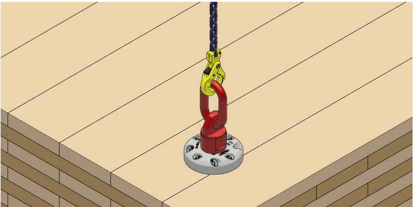
Step 4: Hook in the Powerring at the predetermined angle (see technical data) and lift.
